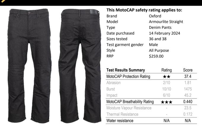
This garment is fitted with impact protectors for the knees and hips. There are no vents to allow airflow movement through the garment. There is the potential for burns from heat transferred through the fly button and pocket studs of the pants during a slide.
