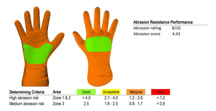
**Individual Abrasion Resistance Results:** - The table below shows the test results for time to abrade through all layers of the materials. Calculated for each sample by Zone, type and area coverage of each material as a proportion of that Zone. Abrasion times are capped at a maximum of 10.00s.
